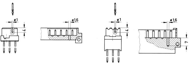
Drill out the male connector at pre-centered point according to the sketch. The coding pin can then be inserted into the corresponding cavity of the female connector by means of the insertion tool. This coding system is available only for the types D, E, F and interface connectors I.
